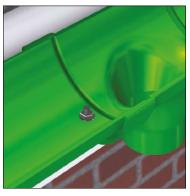
Finger tighten nut and bolt only, pull the joint apart sideways to ensure a minimum 3mm expansion gap is achieved. Then tighten one full turn only, with a spanner or screwdriver.
