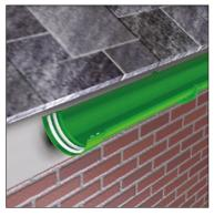
Clean all joint surfaces using a clean cloth and Alutec solvent cleaner, code SC108. Ensure all surfaces are dry and then apply two 8mm parallel beads of Alutec sealant, code SC101 to the gutter socket and around the bolt hole.
