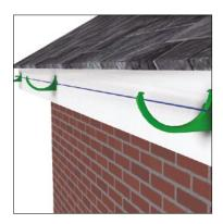
Fix fascia brackets at 915mm centres.For best flow rate, fix to a fall of 1:600 or alternatively nominally level.
