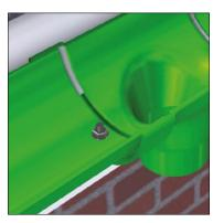
Point sealant onto joint gap, adding additional Alutec sealant, code SC101 if required. Clean off any excess with Alutec solvent cleaner, code SC108.
