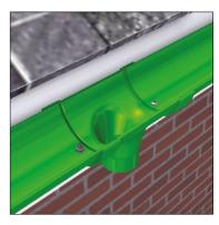
Nuts and washers can be located inside or outside the gutter. Bolt heads outside the gutter will appear neater, but the internally projecting thread will have a minor effect on flow rate performance. Both options are illustrated.
