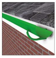
Place gutters into the fascia brackets and press down to engage into fascia brackets. Do not slide the gutter into the fascia brackets, as this may result in the gutter surface being marked.
