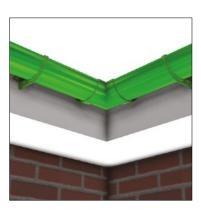
Support all corner angles and outlets by fixing fascia brackets a maximum of 150mm from each side.
