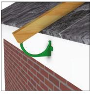
Set gutter height by laying a straight batten on the lowest profile of the roof. Place the fascia bracket under the batten so that they are touching and mark the screw holes.
