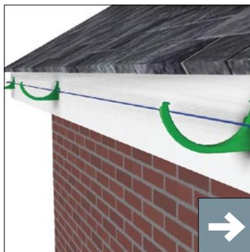
3. Fix fascia brackets at 915mm centres. For best flow rate, fix to a fall of 1:600 or alternatively nominally level.
