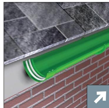
6. Clean all joint surfaces using a clean cloth and Alutec solvent cleaner, code SC108. Ensure all surfaces are dry and then apply two 8mm parallel beads of Alutec sealant, code SC101 to the gutter socket and around the bolt hole.
