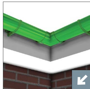
4. Support all corner angles and outlets by fixing fascia brackets a maximum of 150mm from each side.
