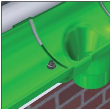
9. Point sealant onto joint gap, adding additional Alutec sealant, code SC101 if required. Clean off any excess with Alutec solvent cleaner, code SC108.
