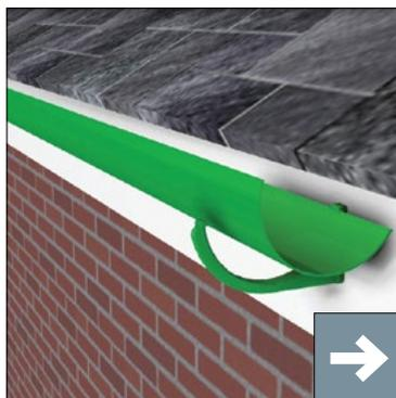
5. Place gutters into the fascia brackets and press down to engage into fascia brackets. Do not slide the gutter into the fascia brackets, as this may result in the gutter surface being marked.
