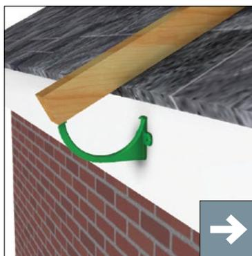
1. Set gutter height by laying a straight batten on the lowest profile of the roof. Place the fascia bracket under the batten so that they are touching and mark the screw holes.
