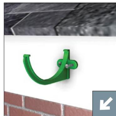
2. Fix fascia brackets with Alutec 32mm x No. 10 roundhead screws, code SC201 or Alutec 15mm x No. 10 countersunk screw, code SC203 if fixing to Alutec aluminium composite fascia. Drilling pilot holes first is recommended.
