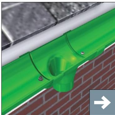
7. Nuts and washers can be located inside or outside the gutter. Bolt heads outside the gutter will appear neater, but the internally projecting thread will have a minor effect on flow rate performance. Both options are illustrated.
