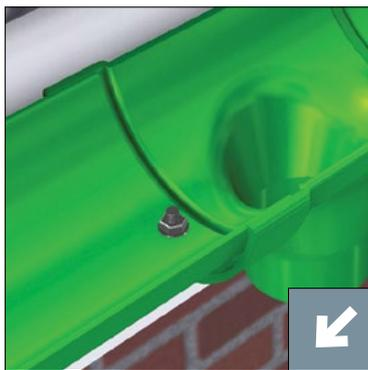
8. Finger tighten nut and bolt only, pull the joint apart sideways to ensure a minimum 3mm expansion gap is achieved. Then tighten one full turn only, with a spanner or screwdriver.
