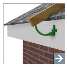
Set gutter height by laying a straight batten on the lowest profile of the roof. Place the fascia bracket under the batten so that they are touching and mark the screw holes.
