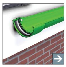
Anchor joint union to fascia board using Marley Alutec No. 10 x 32mm roundhead screws SC201 or Marley Alutec No. 10 x 15mm countersunk screw, code SC203 if fixing to Marley Alutec aluminium composite fascia. Drilling a pilot hole first is recommended.
