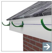
Fix fascia brackets at 1 metre centres. For best flow rate fix to a fall of 1:600 or alternatively nominally level.
