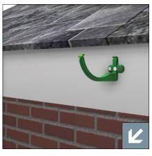
Fix fascia brackets with Marley Alutec No. 10 x 32mm roundhead screws, code SC201 or Marley Alutec No. 10 x 15mm countersunk screw, code SC203 if fixing to Marley Alutec aluminium composite fascia. Drilling pilot holes first is recommended.
