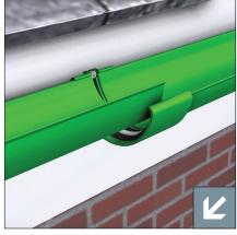
Repeat stages 5 & 6 and joint the gutter length to the one previously fixed. Ensure a 3mm expansion gap is left between the gutter ends.
