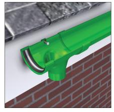
Anchor outlets to fascia board using Marley Alutec No. 10 x 32mm roundhead screws SC201 or Marley Alutec No. 10 x x15mm countersunk screw, code SC203 if fixing to Marley Alutec aluminium composite fascia. Drilling a pilot hole first is recommended.
