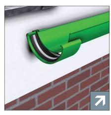
6. Place the gutter into the fascia brackets without clipping the front down. Position the union onto the rear of the gutter then snap the gutter fully into the fascia brackets. Finally apply upward pressure to the union clip from the bottom, whilst pulling the front gutter edge into the union clip.
