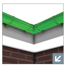
Support all corner angles by fixing fascia brackets a maximum of 150mm from each side.
