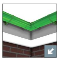
Support all corner angles by fixing fascia brackets a maximum of 150mm from each side.
