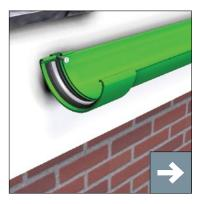
Anchor joint union to fascia board using Alutec 32mm x No. 10 roundhead screws SC201 or Alutec 15mm x No. 10 countersunk screw, code SC203 if fixing to Alutec aluminium composite fascia.
