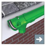
Anchor outlets to fascia board using Alutec 32mm x No. 10 roundhead screws SC201 or Alutec 15mm x No. 10 countersunk screw, code SC203 if fixing to Alutec aluminium composite fascia. Drilling a pilot hole first is recommended.
