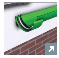
Place the gutter into the fascia brackets without clipping the front down. Position the union onto the rear of the gutter then snap the gutter fully into the fascia brackets.
