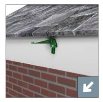
Fix fascia brackets with Alutec 32mm x No. 10 roundhead screws, code SC201 or Alutec 15mm x No. 10 countersunk screw, code SC203 if fixing to Alutec aluminium composite fascia. Drilling pilot holes first is recommended.
