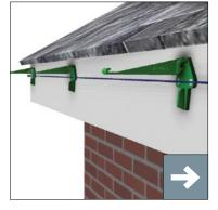
Fix fascia brackets at 1 metre centres. For best flow rate fix to a fall of 1:600 or alternatively nominally level.
