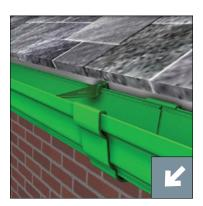
8. Repeat stages 5 & 6 and joint the gutter length to the one previously fixed. Ensure a 3mm expansion gap is left between the gutter ends.
