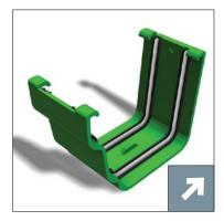
Prior to assembling gutter joints, apply sealant to the central grooves. Use only Alutec sealant, code SC101.
