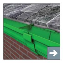
Push the union from below upwards over the gutter, clipping over the rear first, followed by the front of the gutter. Follow the same fitting process for outlets, angles and stop-ends.
