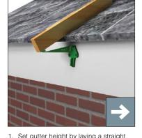
Set gutter height by laying a straight batten on the lowest profile of the roof. Place the fascia bracket under the batten so that they are touching and mark the screw holes.
