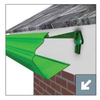
4. Hook the front edge of the gutter into the front of the fascia brackets.
