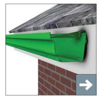
5. Swing the rear of the gutter upwards and engage into the fascia brackets.
