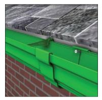
Anchor all fittings to fascia board using Alutec 32mm x No. 10 roundhead screws, code SC201 or Alutec 15mm x No. 10 countersunk screw, code SC203 if fixing to Alutec aluminium composite fascia.
