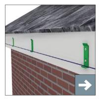
Fix fascia brackets at 750mm centres.For best flow rate, fix to a fall of 1:600 or alternatively nominally level.
