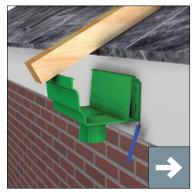
1. Set gutter height by laying a straight batten on the lowest profile of the roof
