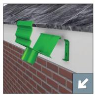
Fix an additional fascia bracket centrally to one side of each angle and centrally to each outlet.
