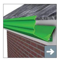
Hook the rear of the gutter over the top of the fascia brackets and then swing down to secure into the base of the fascia brackets.
