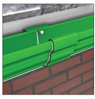
Anchor union to fascia board using Alutec 32mm x No. 10 screw, code SC202 or Alutec 15mm x No. 10 countersunk screw, code SC203 if fixing to Alutec aluminium composite fascia. Ensure a 3-4mm expansion gap is left.
