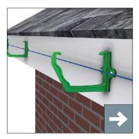
Fix fascia brackets at 1m centres. For best flow rate, fix to a fall of 1:600 or alternatively nominally level.
