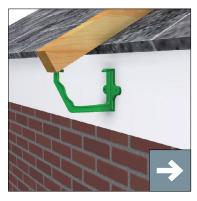
Set gutter height by laying a straight batten on the lowest profile of the roof.
