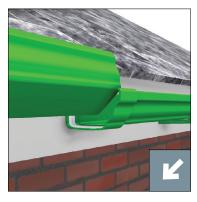
Fit gutter into fascia brackets by inserting the rear upstand, then snapping down the front. Repeat steps 6. 7 & 8.
