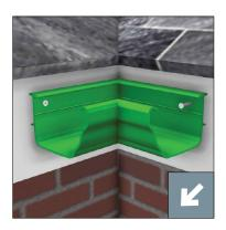
Fix all gutter angles with 2 no. Alutec 32mm x No. 10 countersunk screw, code SC202 or Alutec 15mm x No. 10 countersunk screw, code SC203 if fixing to Alutec aluminium composite fascia.
