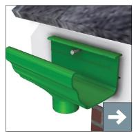
Position outlets and fix using Alutec 32mm x No. 10 countersunk screw, code SC202 or Alutec 15mm x No. 10 countersunk screw, code SC203 if fixing to Alutec aluminium composite fascia
