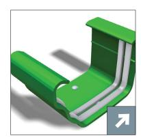
Ensure the factory fitted rubber compression spacers are attached to the inside of the union. Clean all joint surfaces using a clean cloth and Alutec solvent cleaner, code SC108. Ensure all surfaces are dry and then apply two 8mm parallel beads of Alutec sealant, code SC101 to each side of the union.
